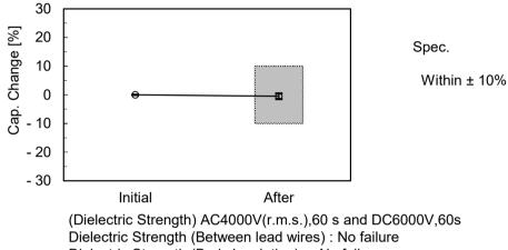
Dielectric Strength (Between lead wires) : No failure Dielectric Strength (Body Insulation) : No failure Insulation Resistance (I.R.) :  $1000M\Omega$  min. Appearance : No marked defect
